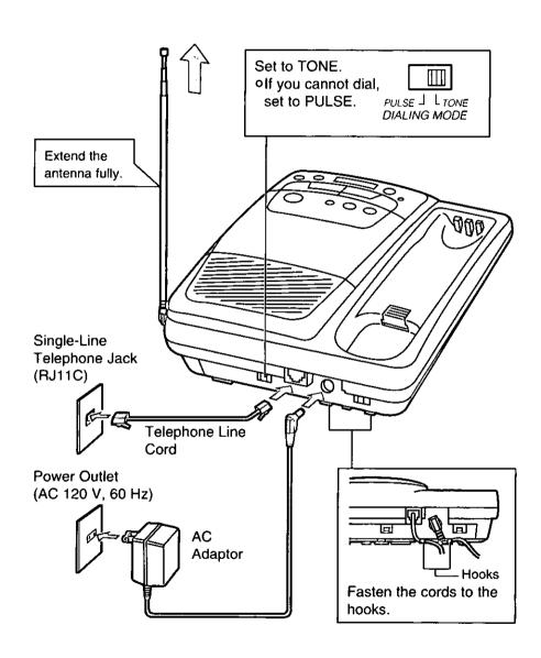
**OUSE ONLY Panasonic AC ADAPTOR KX-A11.** •The AC adaptor must remain connected at all times. (It may feel warm during use. This is normal.)
